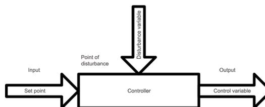
Figure 1: Controlled system
