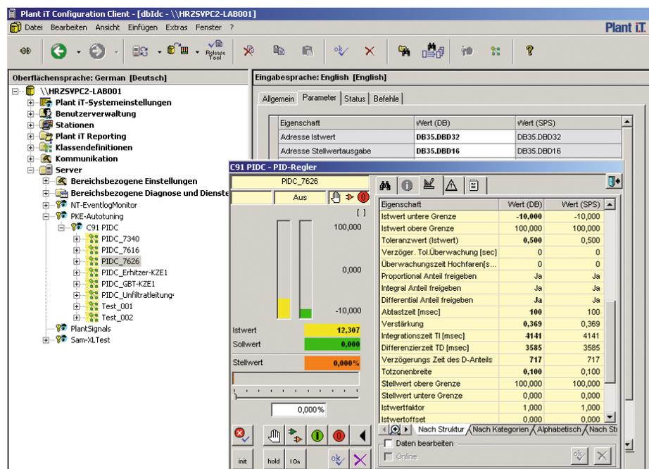
Figure 4: Integrated in the process control systems Plant iT/brewmaxx
