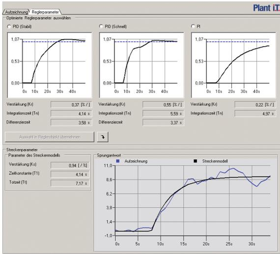
Figure 5: Comparative view of the controller parameters
