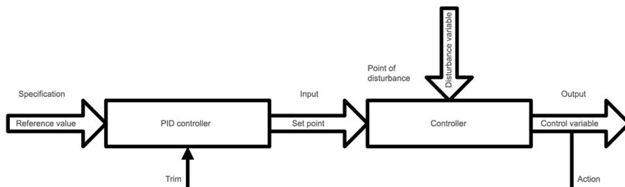
Figure 2: Controlled loop
