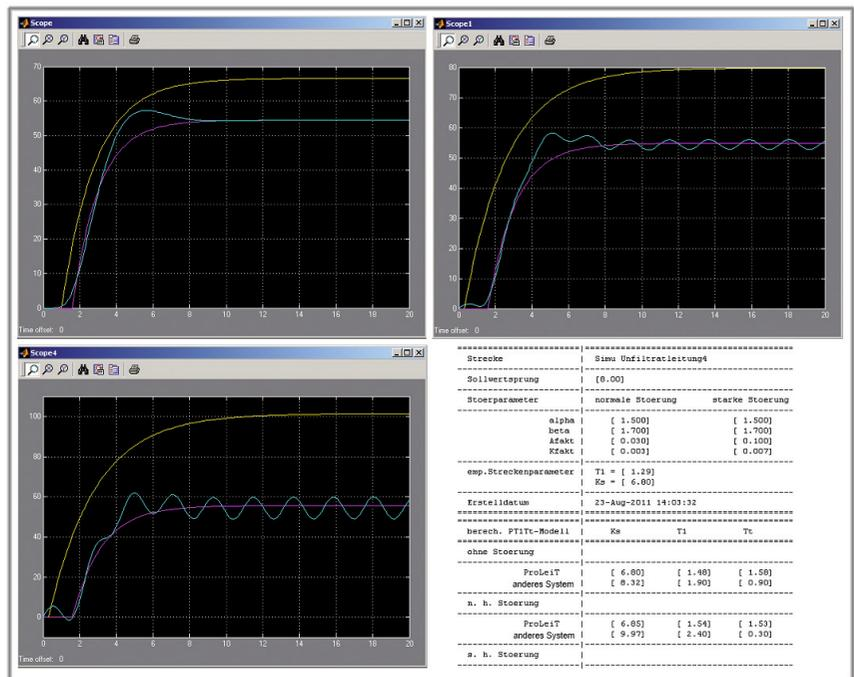
Figure 6: Comparative test – optimum controlled system with the new autotuning function from ProLeiT
