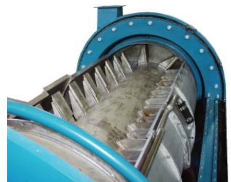
Fig. 1 TR dry cleaner – screen cage open, view of the rotor and paddle
