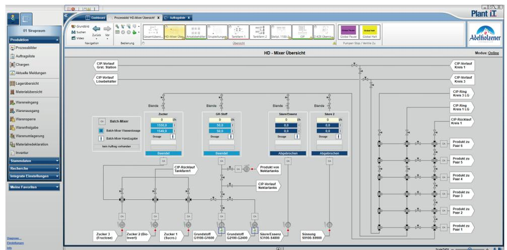
Plant Batch iT – process image of the batch mixer
